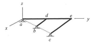
(c) A two-member structure abc is connected by a pin at c and supported by hinges at a and b. Neglect the thickness of the members. (6%)
